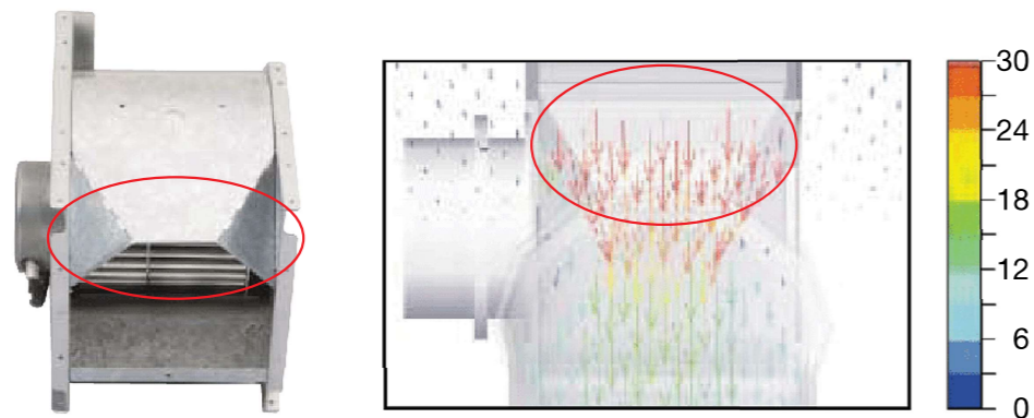
Internal Wind Velocity Distribution – Airflow Analysis
